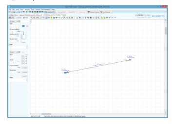
Fluid data: Gasoline with a 0.736 specific gravity and 0.6 cSt viscosity.
