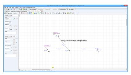
Fluid data: Natural Gas with specific gravity 0.60 (0.046 lb/ft³), 60 °F, 0.00 kPa.g, viscosity 0.0119 centipoise.
