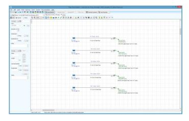
Fluid data: Air at 100 psi gauge and 60°F, density 0.595574 lb/ft<sup>3</sup>, viscosity 0.018095 centipoise.
