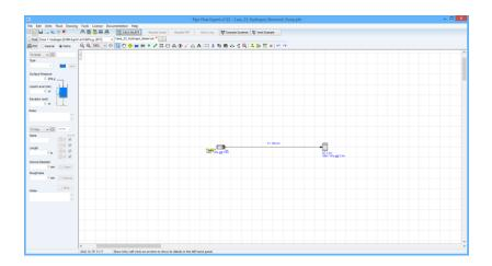
Fluid data: Hydrogen at 21.85 °C, 0.0 bar.g, density 0.084 kg/m³, viscosity 0.009 centipoise.
