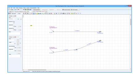
Fluid data: Natural Gas with specific gravity 0.6, 60 °F, 14.696 psi.g (0.04582 lb/ft³), viscosity 0.01191 centipoise.
