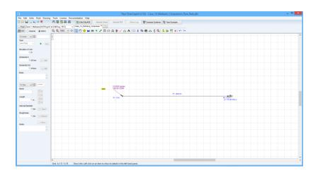
Fluid data: Methane at 293 K average, 0.00 kPa.g, density 0.667218 kg/m³, viscosity 0.0108 centipoise.
