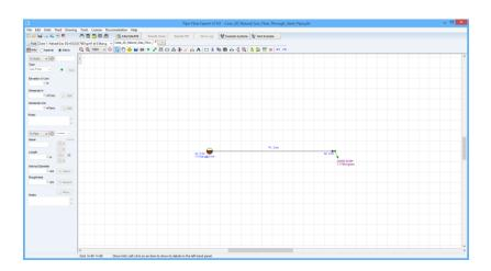
Fluid data: Natural Gas at 15 °C, specific gravity 0.62, 0.0 bar.g, density 0.760 kg/m<sup>3</sup>, viscosity 0.0120 centipoise.
