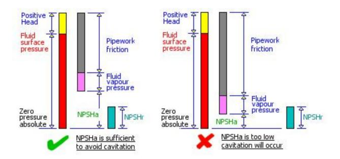
In a system where the fluid needs to be lifted to the pump inlet, the negative head reduces the motive force to move the fluid to the pump.
